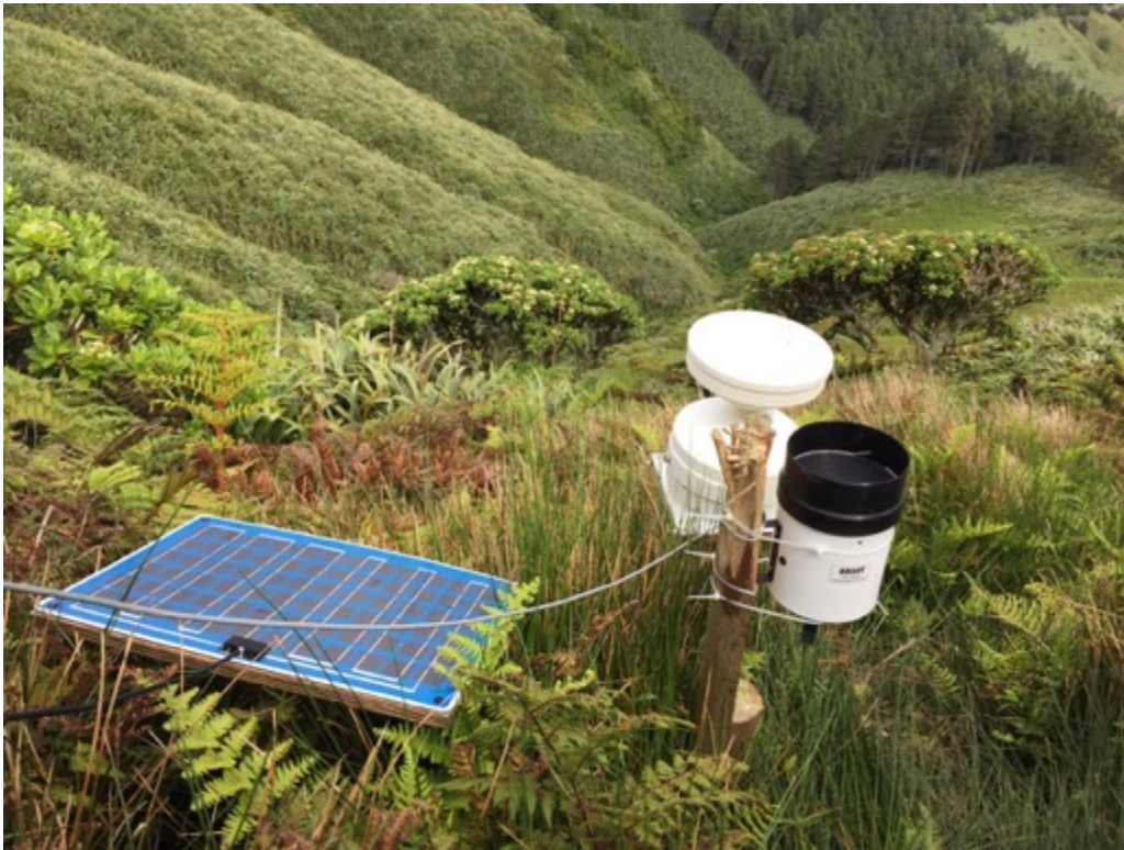
Plate 3.2: Rain gauge at Grapevine Gut
